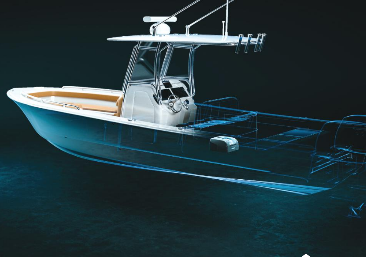
A Seakeeper 1 in a 26-foot center console is shown here, to scale.
