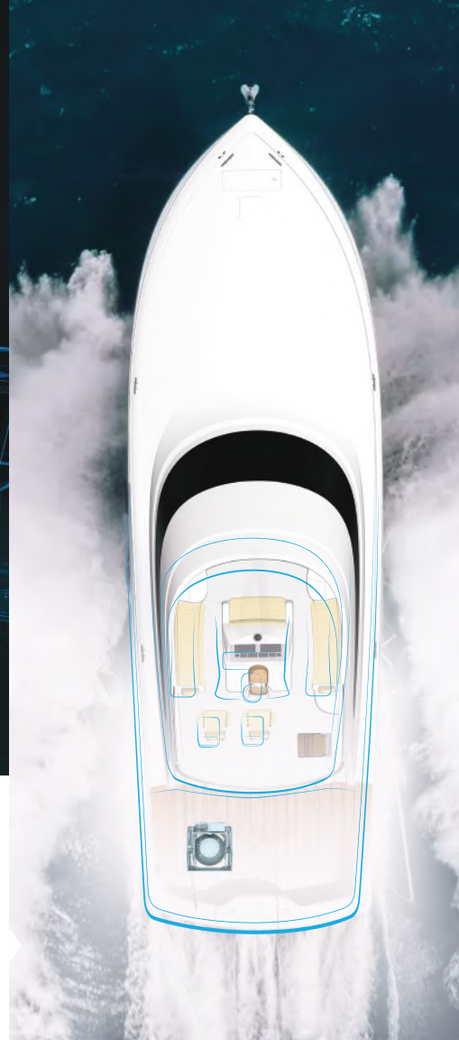
A Seakeeper 1 in a 26-foot center console is shown here, to scale.
