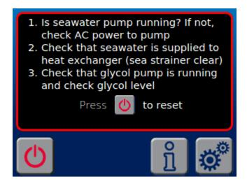
• To reset the ALARM utilize the Seakeeper ON/OFF button
