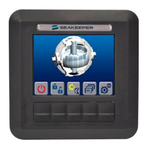
FIGURE 4 - OPERATOR DISPLAY
