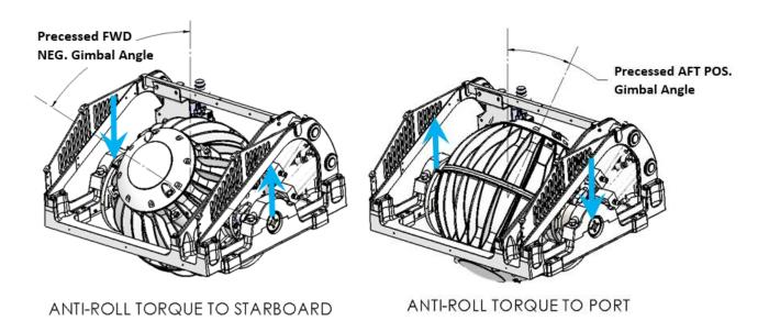
FIGURE 2 – SEAKEEPER PRECESSION
