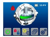
3) Press Seakeeper ON/OFF button. The ON/OFF symbol will turn RED. The Seakeeper will start coasting.
