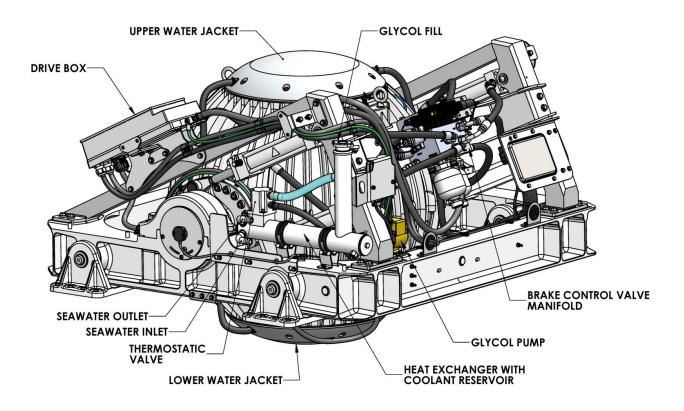
FIGURE 7 – COOLING SYSTEM COMPONENTS
