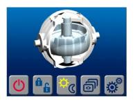
To turn the Seakeeper ON depress the POWER ON/OFF FAULT RESET button, the button will turn GREEN, the flywheel will spin (or arrow appear), and a RED PROGRESS BAR will appear. The PROGRESS BAR indicates how soon the Seakeeper will be available for stabilization. When the Seakeeper is initialized and up to minimum operating speed the PROGRESS BAR will turn from RED to GREEN. At this point, the Seakeeper is available for stabilization.
