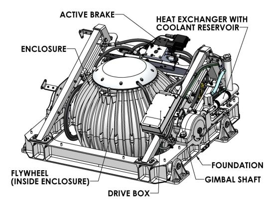
FIGURE 3 - SEAKEEPER ASSEMBLY
