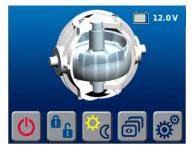
4) Once the vessel is secured in the slip and the crew has shut down the generator and engines, switch the AC and DC breakers that control the Seakeeper OFF. The flywheel will continue to spool down to zero rpm. This can take 4.5+ hours from full speed.
