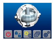
3) The DISPLAY has a set of five buttons that are under the BUTTON ICONS that appear on the display screen. The BUTTONS are the means for selecting the functions of the DISPLAY.
