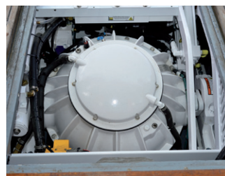
Here the gyro is preceding forward, thereby countering roll to the starboard side.
