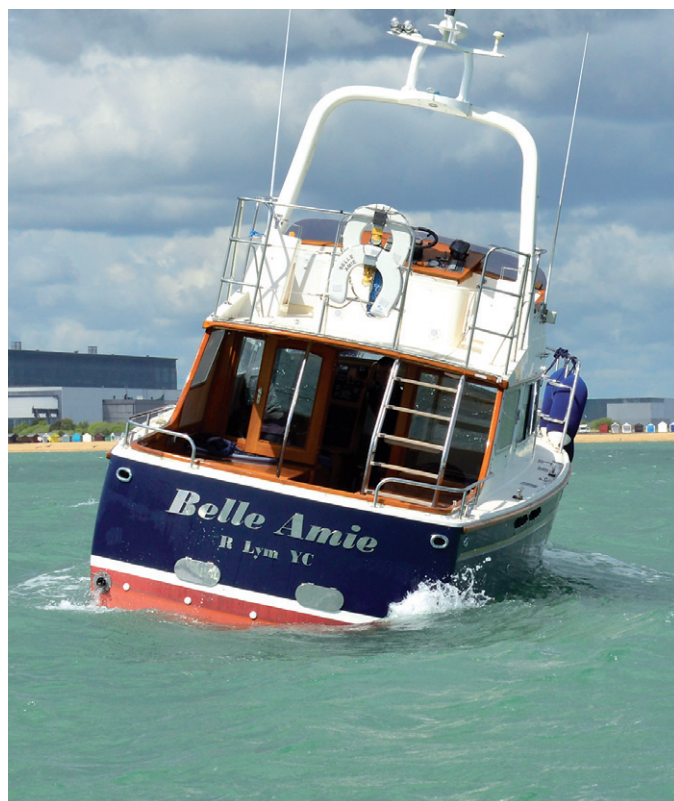
SEAKEEPER 5 OFF - With the gyro locked, the Hagg 36 immediately starts to roll.
