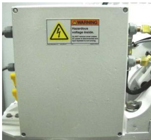
FIGURE 6 – COMPACT MOTOR DRIVE BOX MOUNTED ON FRAME, 3 VIEWS
