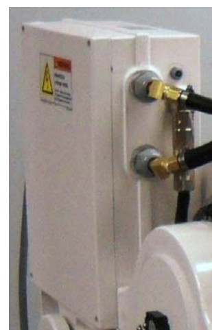
FIGURE 6 – COMPACT MOTOR DRIVE BOX MOUNTED ON FRAME, 3 VIEWS
