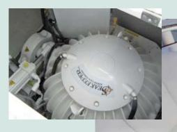
The Seakeeper gyro unit tucks away under a forward hatch in this Intrepid 390. Expect to see more installations of these units on fishing boats at the fall boat shows.
