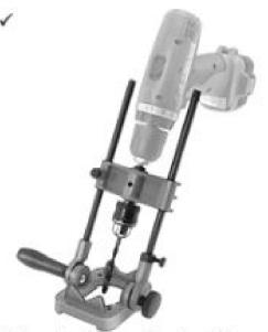
Drill precise holes without a drill press. Simply attach the chuck on your 3/8" or 1/2" capacity portable drill to the drill guide's drive spindle. A dual-locking knob and handle with an easy-to-read protractor let you position your drill up to 45° in either direction. Guides have a built-in V-groove that centers round material up to 2 1/2"
