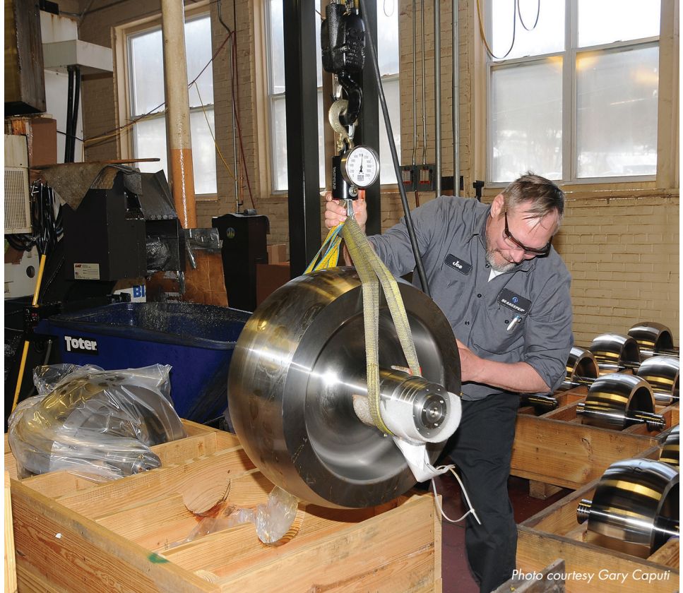
A Seakeeper's flywheel is forged of a single piece of stainless steel. Spinning at high rates of speed within the housing, the flywheel creates the unit's torque.
