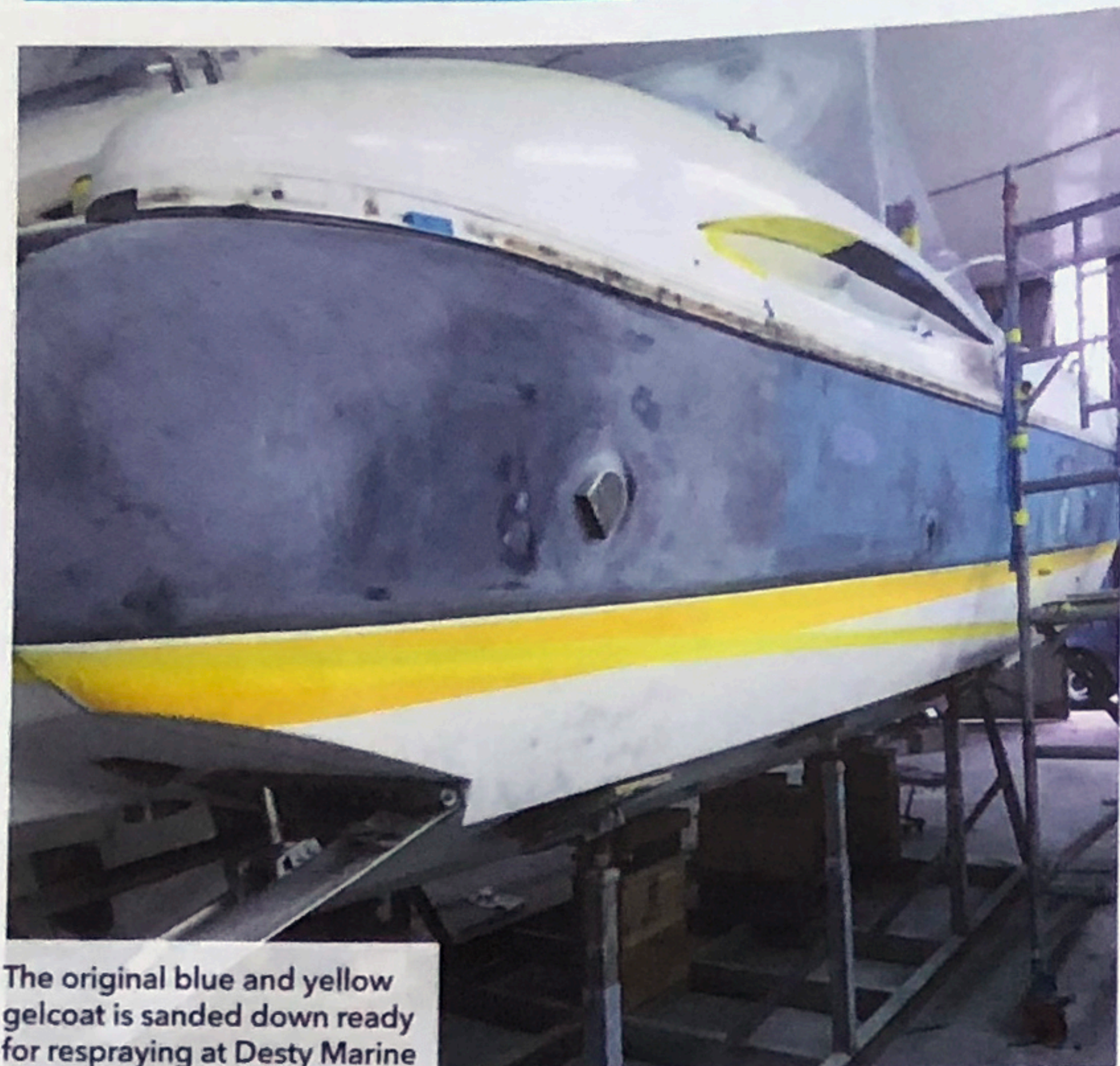
The old antifouling was stripped off and the hull filled and faired for Coppercoating
