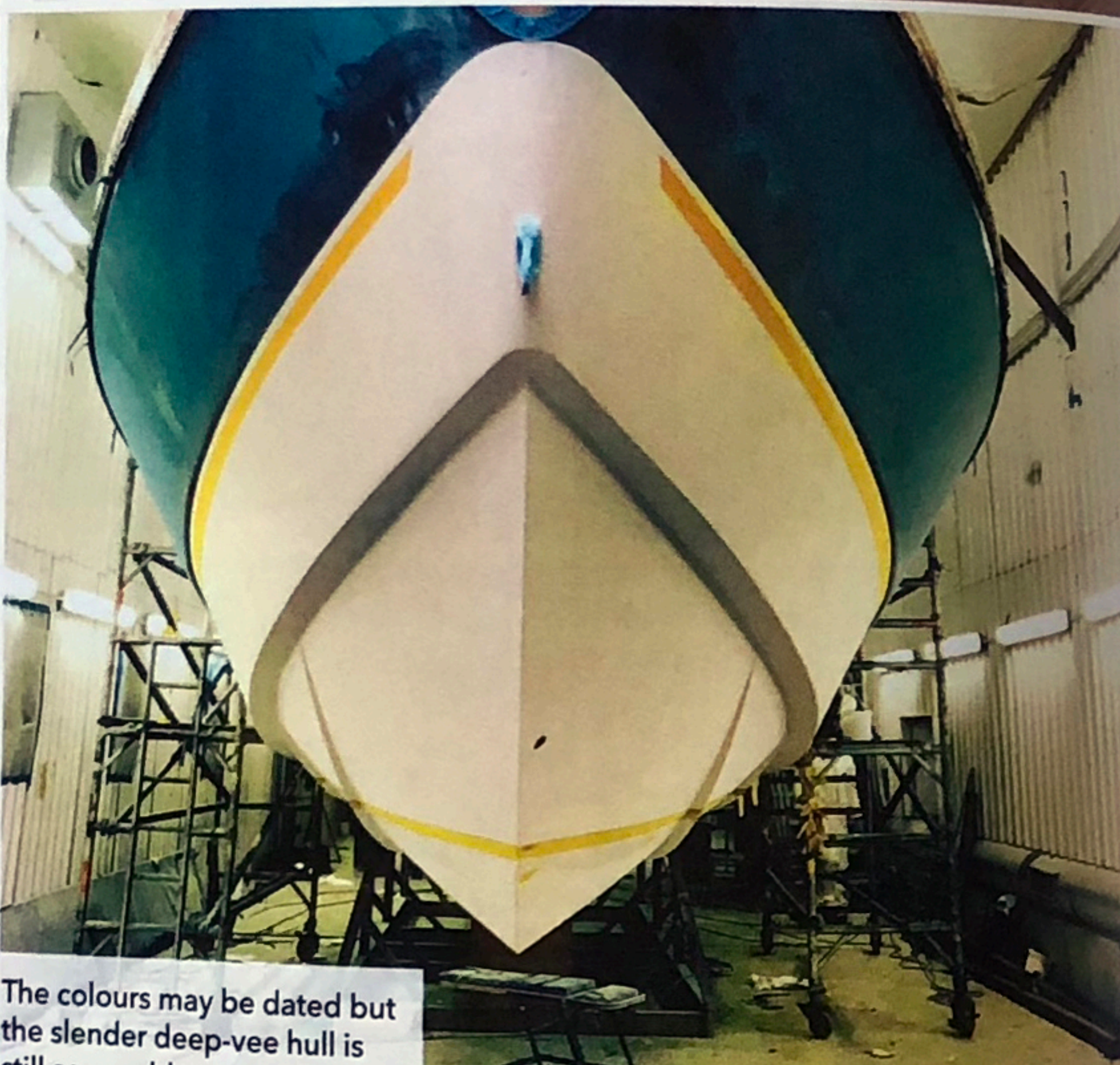
The old antifouling was stripped off and the hull filled and faired for Coppercoating
