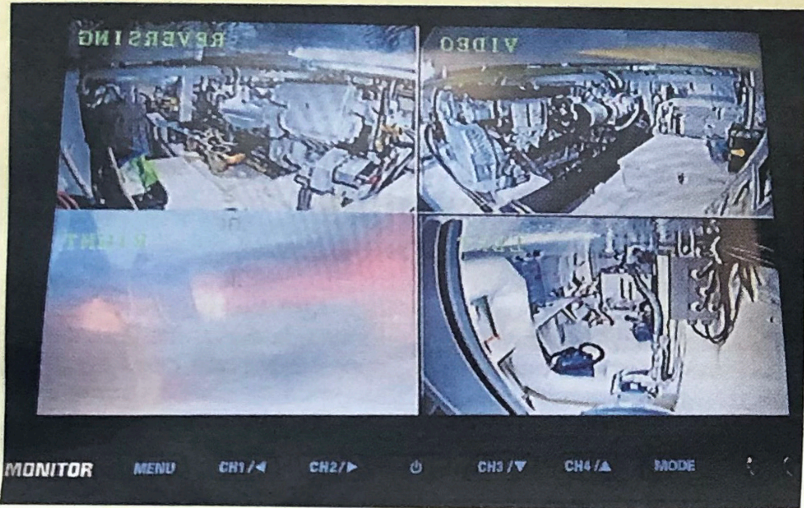
▲ The split-screen CCTV display in the overhead console includes imagery from the underwater camera monitoring the propeller and rudder.
