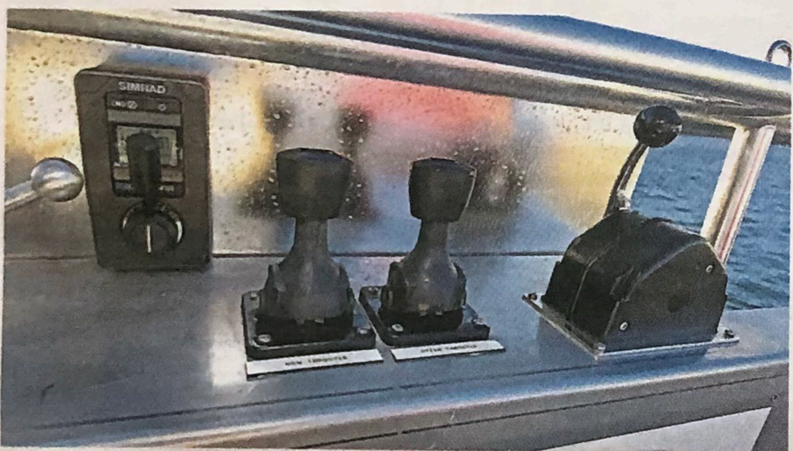
▲ Controls for the hauler, steering, bow/stern thrusters and engine, mounted on the gunwale rail abaft the hauling station, are well-protected.
