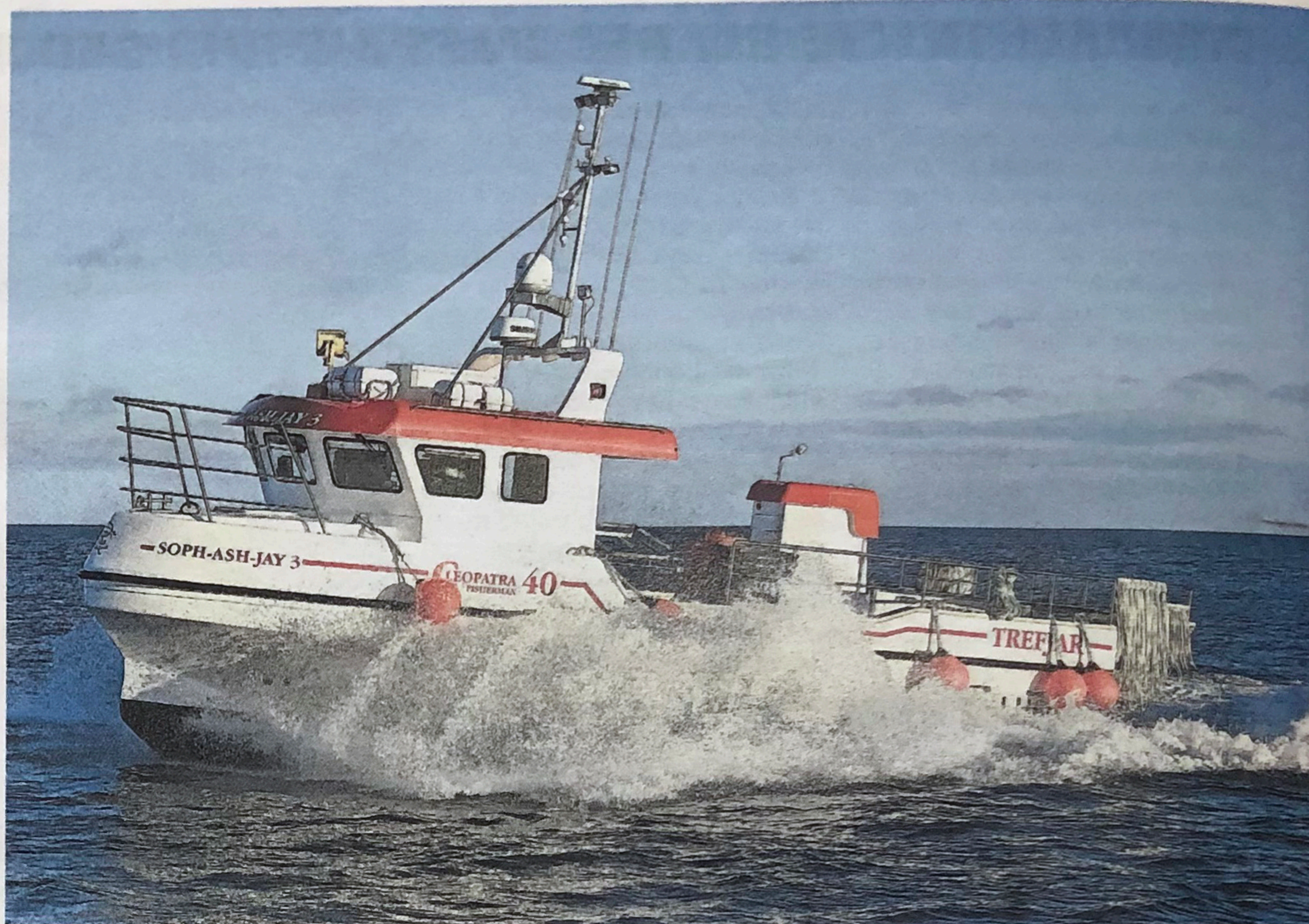
▲ Soph-Ash-Jay 3 has a cruising speed of 12-14 knots, and a top speed of over 20 knots.
