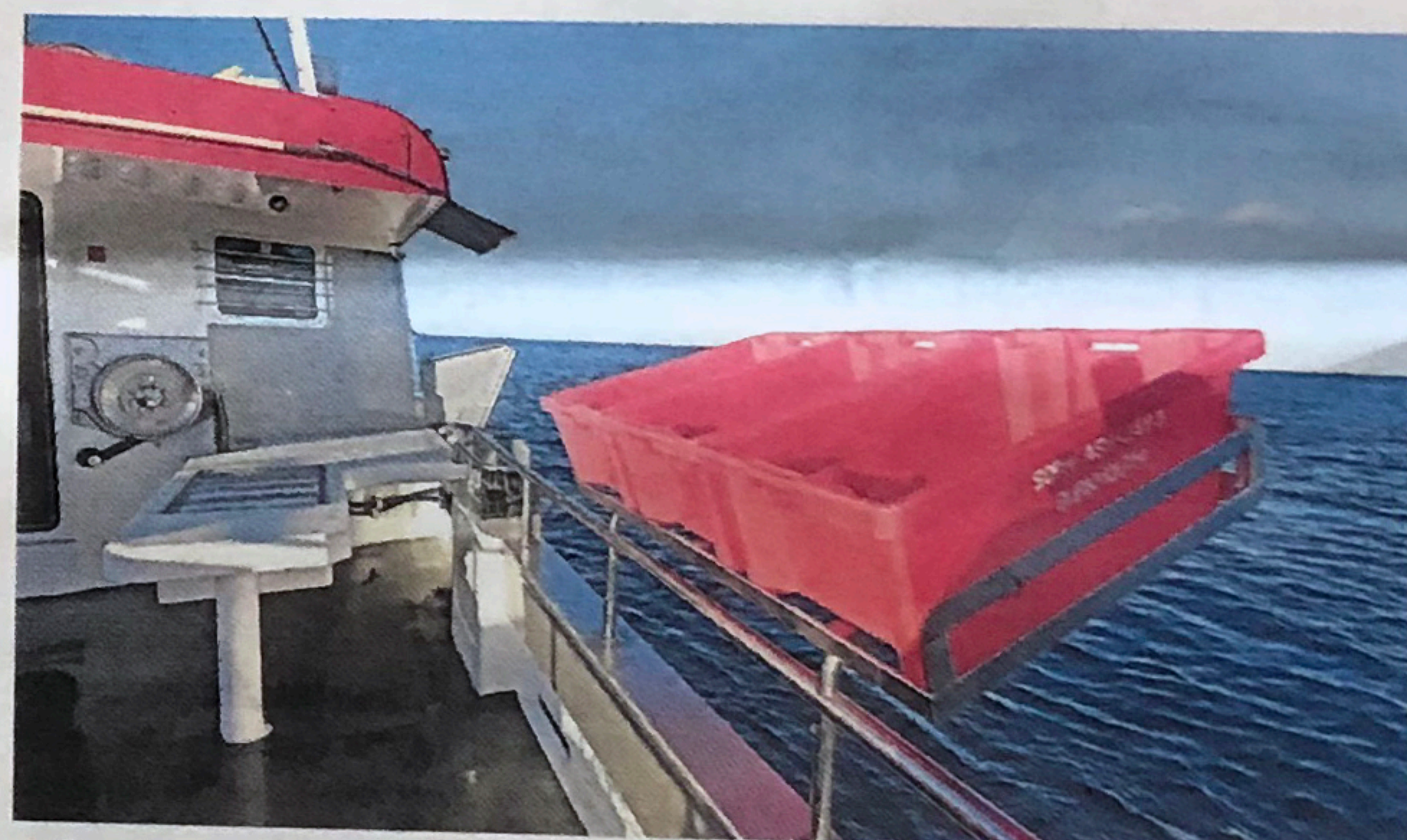
▲ Brown crab are selected in line with market requirements into three fish boxes placed on a secure storage rack abaft the clearing table.
