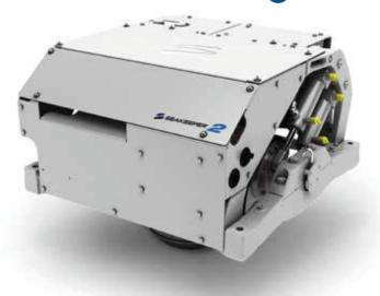
to less than plus to minus 1 degree of roll. This translates to over a 90 percent roll reduction with the Seakeeper 2 unit activated.
