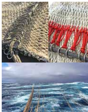
▲ SNG's new wide mackerel brails, incorporating Dynlce bands of netting and Swan-Lock handles, are delivering 'superb quality' fish.
