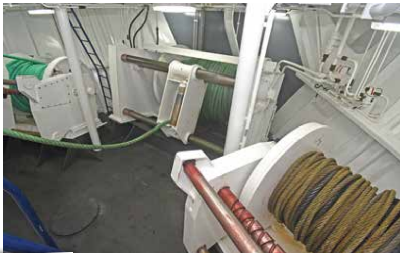
▲ Three 18/24t split trawl winches are fitted in a dedicated room forward...
