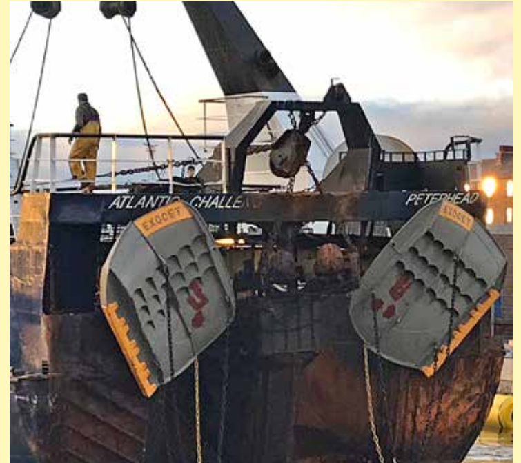
▲ A set of Morgère Exocet trawl doors in use on the Peterhead stern trawler Atlantic Challenge.
