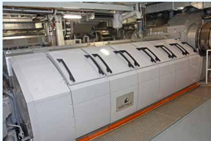
▲ The Wärtsilä 12V31 main engine on the Shetland midwater trawler Research is recognised by Guinness World Records as being the world's most efficient four-stroke diesel engine.
