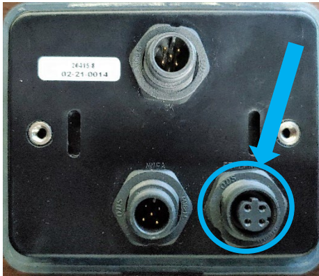
Figure 5: Port for Seakeeper ConnectBox to MFD Connection
