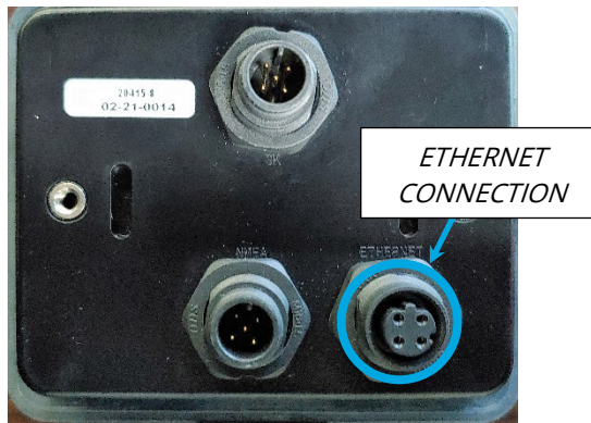
Figure 6: Port for Seakeeper ConnectBox to MFD Connection
