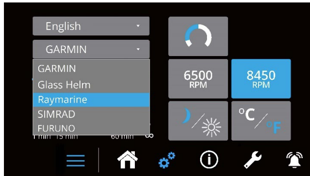
Figure 4: Seakeeper Display's Settings Screen showing Raymarine in the MFD dropdown menu
