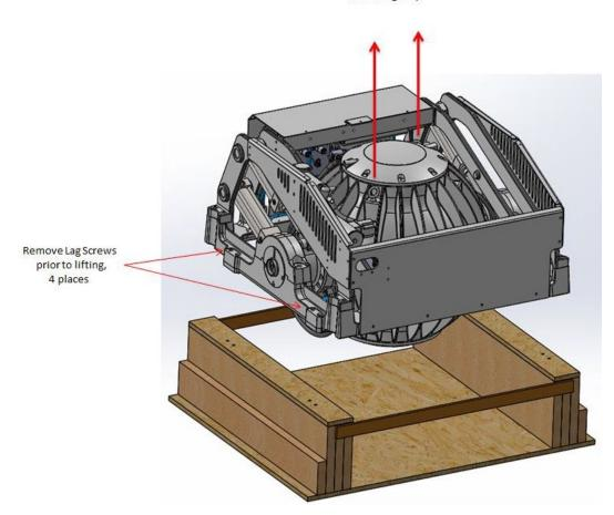
10. **LIFT** Seakeeper per step 8 to place in vessel.
