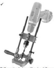
Drill precise holes without a drill press. Simply attach the chuck on your 3/8" or 1/2" capacity portable drill to the drill guide's drive spindle. A dual-locking knob and handle with an easy-to-read protractor let you position your drill up to 45° in either direction. Guides have a built-in V-groove that centers round material up to 2 1/2"
