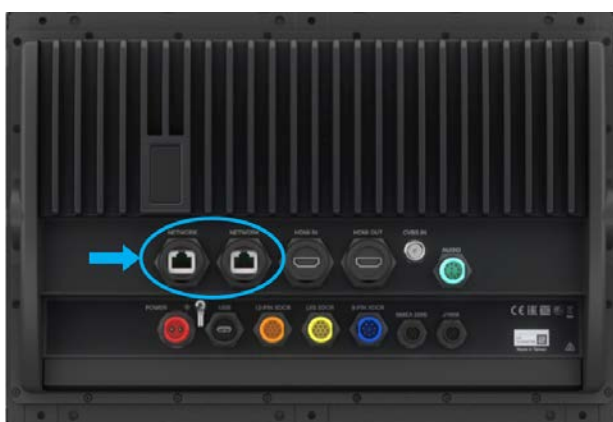
Figure 7: Connect Cable 20373 to a "Network" Port on the Back of the MFD
