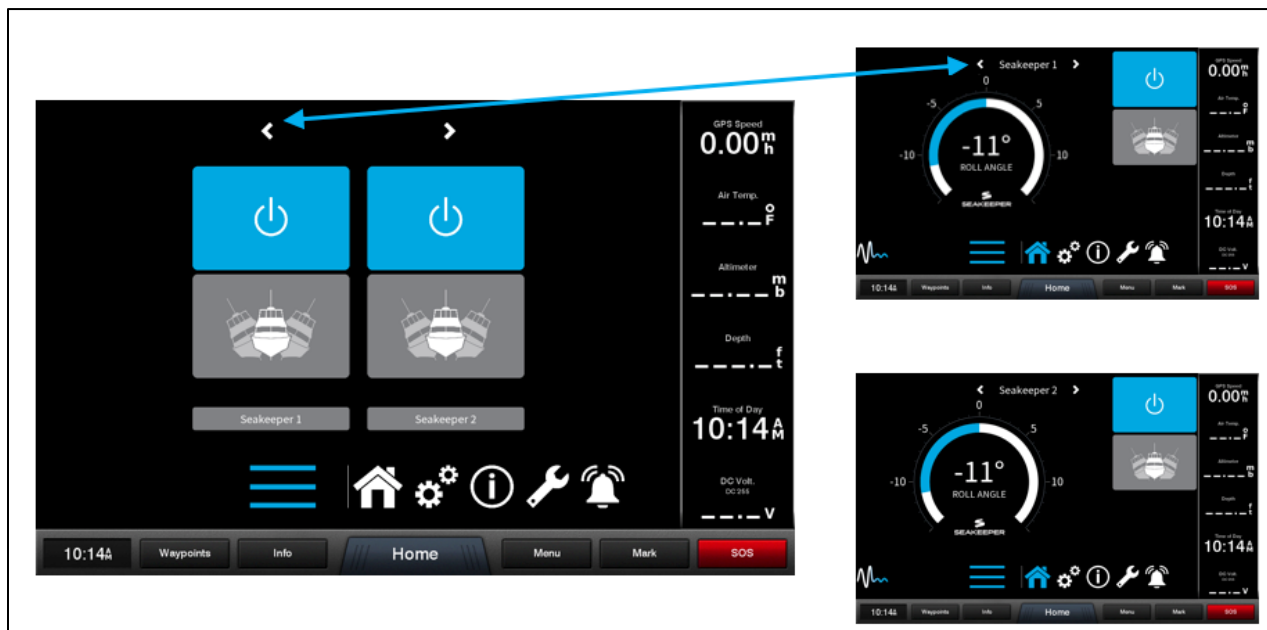
Figure 10: Multi-Seakeeper Home Page (left) Showing Seakeeper Toggle Arrows. Seakeeper 1 Home Page (top right). Seakeeper 2 Home Page (bottom right)
