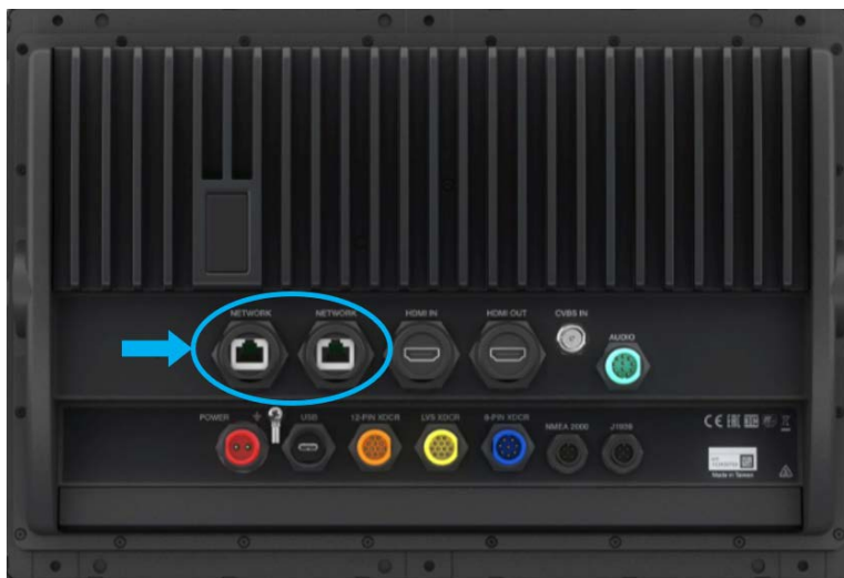
Figure 3: Connect Cable 20373 to a "Network" Port on the Back of the MFD
