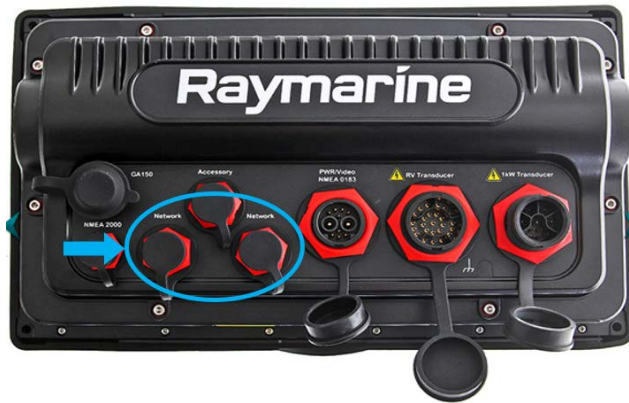
Figure 7: Connect Cable 20380 to a "Network" Port on the Back of the MFD
