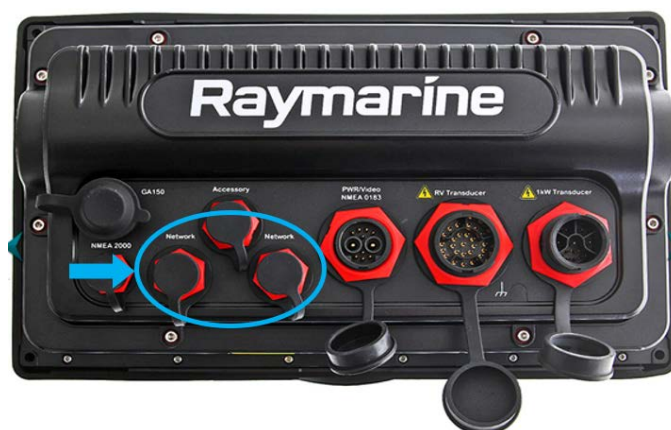
Figure 3: Connect Cable 20380 to a "Network" Port on the Back of the MFD
