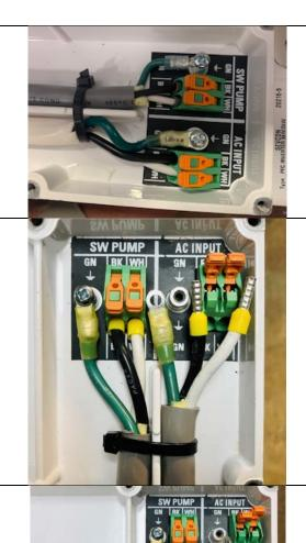
9. Cut cable ties securing AC Power Cable.
