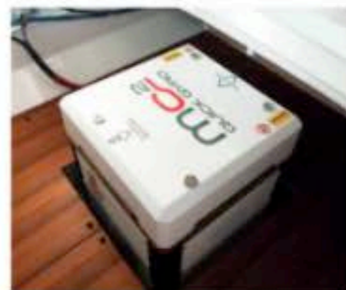
Quick Spa's new MC2 Quick Gyro X2 is aimed at smaller centre-console craft and is air cooled and 12V powered
