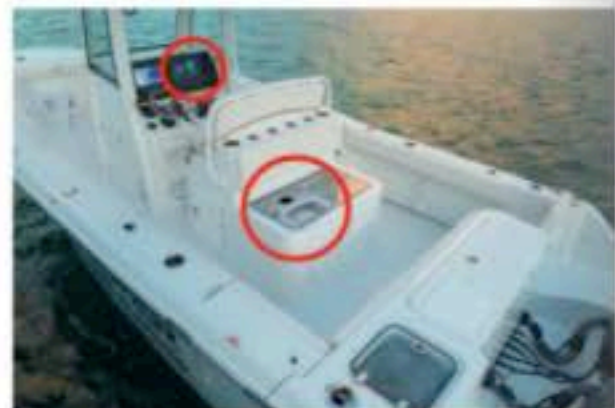
The new Seakeeper 1 typifies a trend for ever more compact units that offer gyro-assisted roll reduction on boats as small as 23ft. This type of unit is air-cooled and runs off a 12V DC battery supply. Note the small size of the unit behind the seat and the large and easily-read display (both circled)
