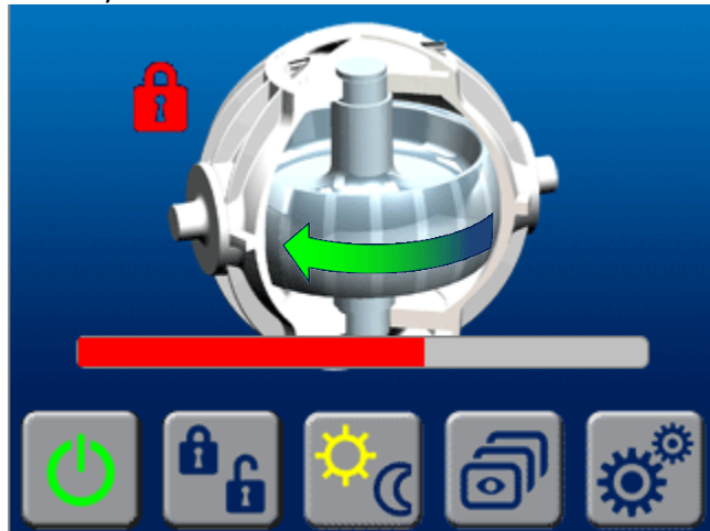
b. Mode 1 – System On – display progress bar showing spool up status – ‘Unlock’ and ‘Lock’ commands not available during early spool up
