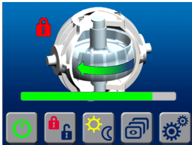
c. Mode 3 – System On and Locked – display progress bar until it reaches 100% – ‘Unlock’ and ‘Lock’ commands are available because the gyro is near operating speed
