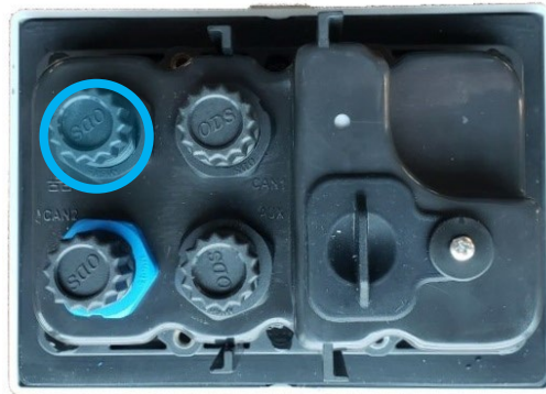
Figure 3: Port for Seakeeper 5" Touch Display to MFD Connection
