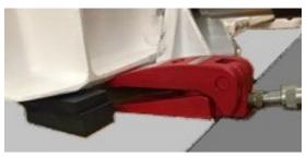
5. <u>IF</u> clevis will not separate from stringer using hydraulic jack, <u>THEN</u> APPLY additional pressure using supplied nut and bolt.
