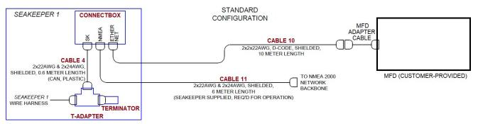
This is supported by the fact that when a 5" display is installed at the Seakeeper onto the gyro CAN network (not the NMEA network) the display works. Removing the 5" display and reconnecting the MFD works for an undetermined time before the MFD again displays Code 251. The Cable 4, Terminator (resistor), T-Adapter, or ConnectBox port is suspect in this event.
