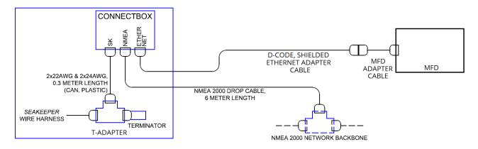
The possible fault is supported by the fact that when a 5" display is installed at the Seakeeper onto the gyro CAN network (not the NMEA network) the display works. Removing the 5" display and reconnecting the MFD works for an undetermined time before the MFD again displays Code 251.The Cable 4, Terminator (resistor), T-Adapter, or ConnectBox port is suspect in this event.
