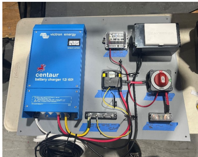
Figure 3: Seakeeper Electrical Panel with Charger
