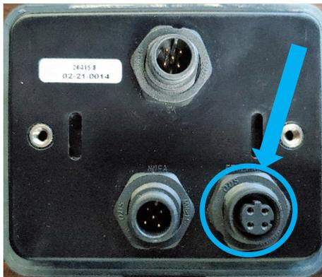
Figure 5: Port for Seakeeper ConnectBox to MFD Connection
