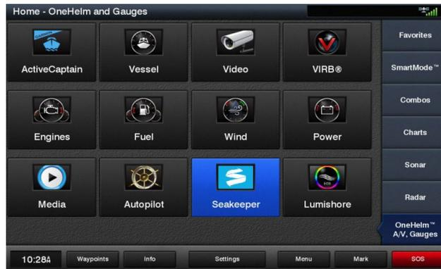
Figure 4: Garmin OneHelm Display – with Seakeeper Application Icon
