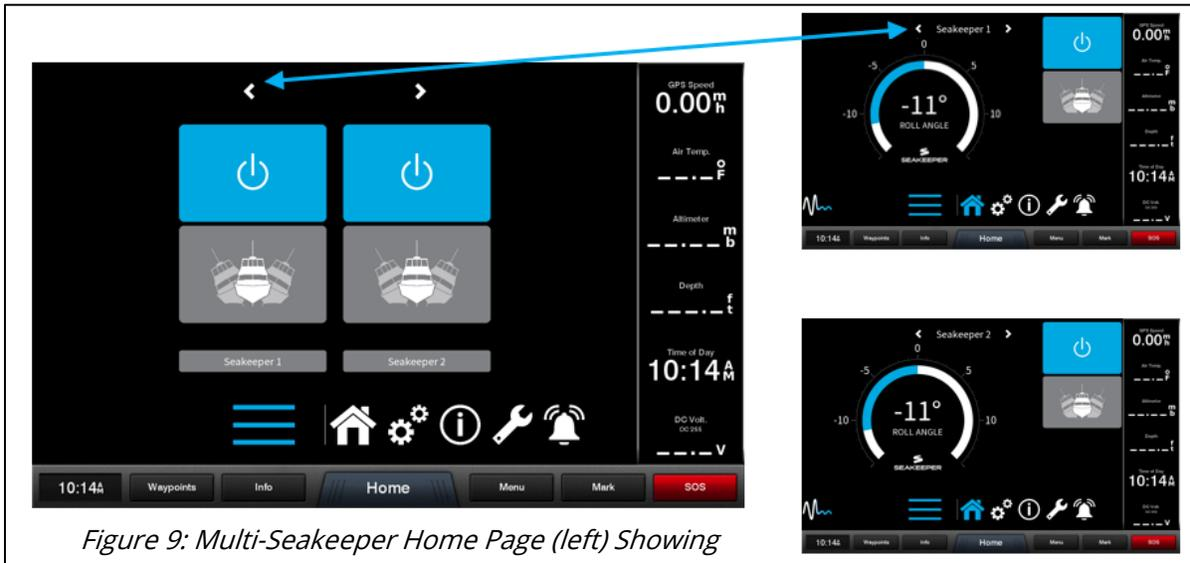
Figure 9: Multi-Seakeeper Home Page (left) Showing Seakeeper Toggle Arrows. Seakeeper 1 Home Page (top right). Seakeeper 2 Home Page (bottom right)
