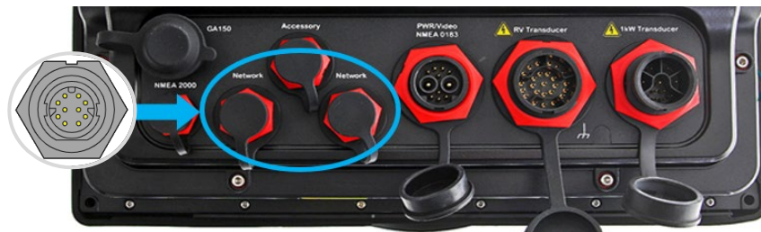
Figure 3: Connect Cable 20380 to a "Network" Port on the Back of the MFD
