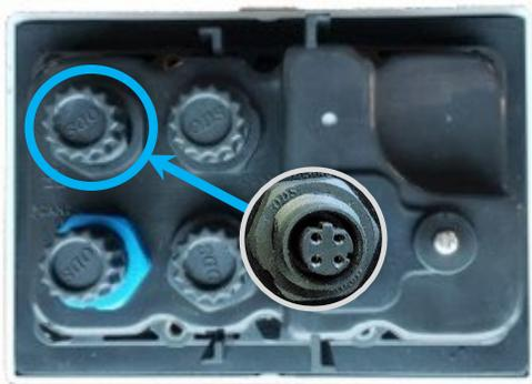
Figure 2: 5" Touch Display Ethernet Port
