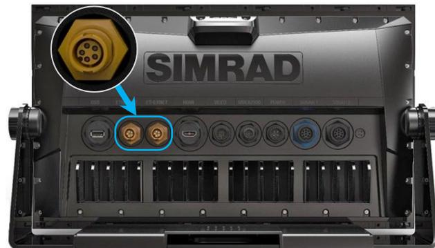
Figure 3: Connect Cable 20346 to "Network" Port
