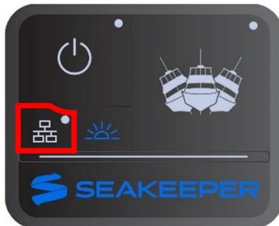
PRESS ETHERNET BUTTON FOR 5-7 SECONDS
