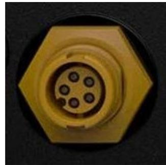
Figure 7: NAVICO ethernet port
