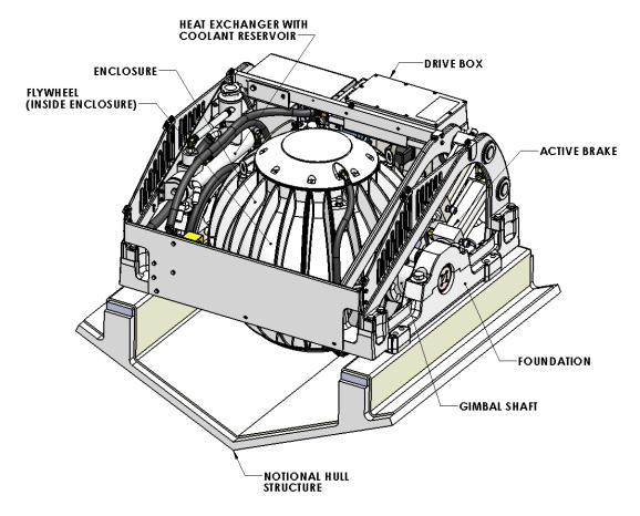
FIGURE 3 - SEAKEEPER ASSEMBLY
