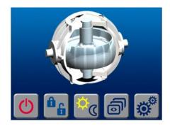
To turn the Seakeeper ON depress the POWER ON/OFF FAULT RESET button, the button will turn GREEN, the flywheel will spin (or arrow appear), and a RED PROGRESS BAR will appear. The PROGRESS BAR indicates how soon the Seakeeper will be available for stabilization. When the Seakeeper is initialized and when the Seakeeper is up to minimum operating speed the PROGRESS BAR will turn from RED to GREEN. At this point, the Seakeeper is available for stabilization.
