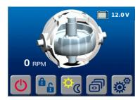
4) Once the vessel is secured in the slip and the crew has shut down the generator and engines, switch the AC and DC breakers that control the Seakeeper OFF. The flywheel will continue to spool down to zero rpm. This can take 4+ hours from full speed.
