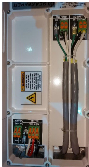
Early Seakeeper 5 through 16, 26, and 35 MDB shown with SW PUMP cable
