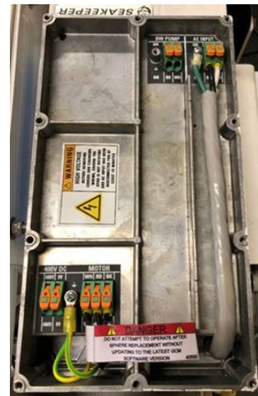
Seakeeper 4.5 through 18, and 40 MDB shown with no SW PUMP cable
