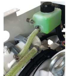
Example of early Seakeeper 2/3 integrated heat exchanger / reservoir
