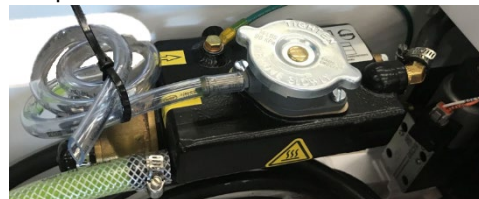
Example of early Seakeeper 2/3 integrated heat exchanger / reservoir
