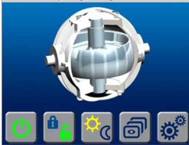
Home Screen with Animation: Flywheel will be spinning and Seakeeper stabilizing
