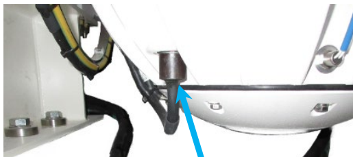
view of feed-through at bottom of enclosure.
