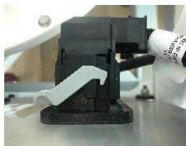
Properly connected GCM 70-pin connector
