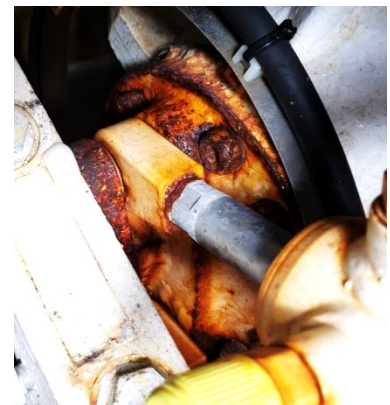
Seakeeper with severe corrosion at rod end clevises, pins, and gimbal shafts
