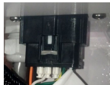
Seakeeper 4.5 MDB connector securely fastened.
