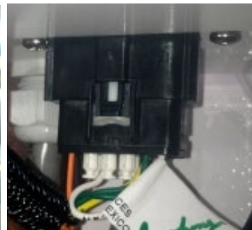
Molex Connector of an Seakeeper 4.5 shown with white locking tab fully inserted
