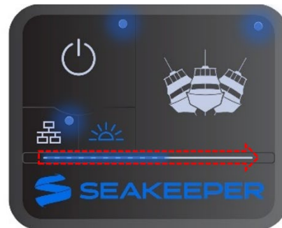
SPOOL BAR LEDs WILL STROBE FROM LEFT TO RIGHT. ROUND LEDs WILL FLASH
