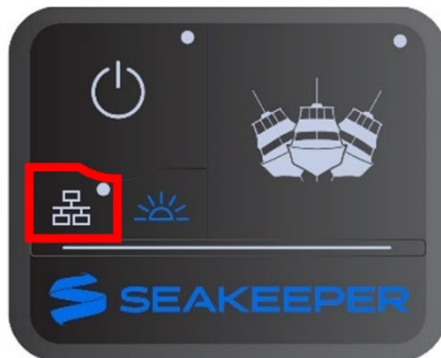
PRESS ETHERNET BUTTON FOR 5-7 SECONDS
