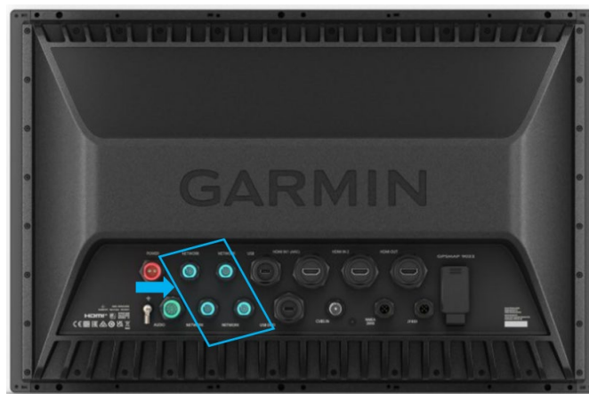
Figure 8: Connect Garmin Cable 010-13094-00 to a "Network" Port on the Back of the 9000 Series MFD
