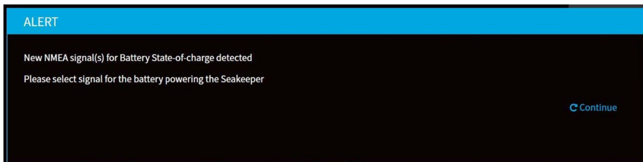
Figure 3: Alert pop-up indicating the SoC signal present on NMEA2000 network.
