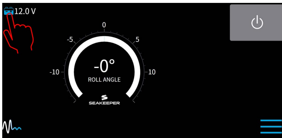
Figure 2: Accessing Battery Monitoring Configuration – Standard method
