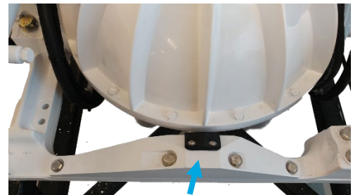
Figure 4: A bump stop of a Seakeeper 5, located at front of foundation.
