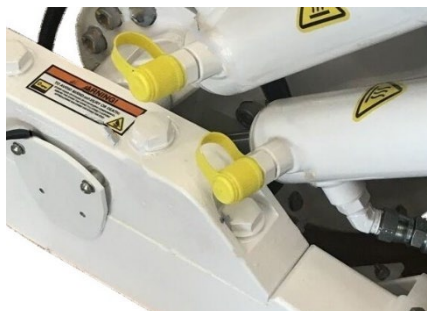
Figure 1: Seakeeper 3 Gimbal Bearing Cap interference by cylinder bleed ports
