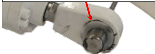
Figure 14: Delrin plastic washer is held to rod-end of cylinder with grease and aligned using brake pin.
