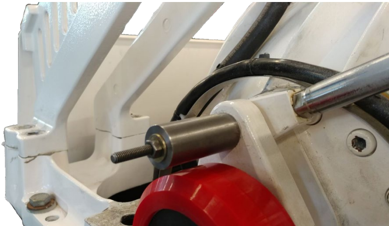
Figure 8: Puller from bushing service kit installed on a rod-end pin
