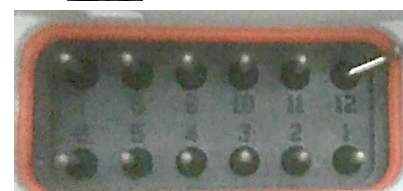
Example of a bent pin found on an IMU.
