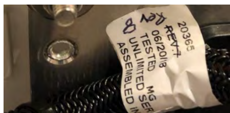
Seakeeper 2 harness should be Rev. 8 or later.
