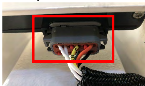
Fully seated IMU connector
