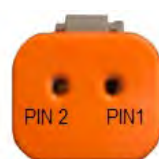
Deutsch connector to prop solenoid from wire harness
