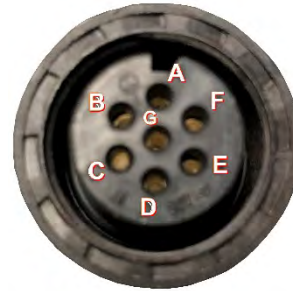
Proportional Brake valve connector for Seakeeper 26, 35, and 40.
