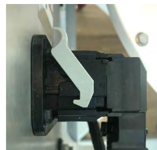
GCM connector fully inserted and locked
