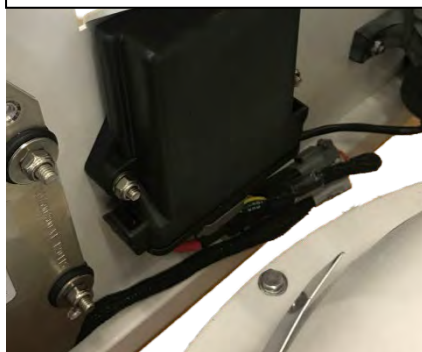
IMU properly installed in a Seakeeper 3
