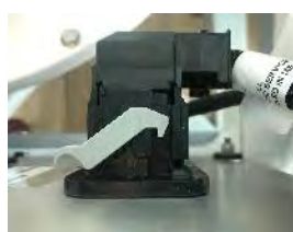
A properly connected GCM 70-pin connector
