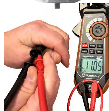
Meter in this photo is displaying 11.05 KΩ.
