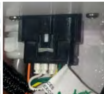
Molex Connector of an AC-powered Seakeeper shown with white locking tab fully inserted
