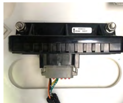
Seakeeper 18/16 IMU shown inside rear panel
