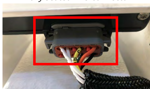
Fully seated IMU connector
