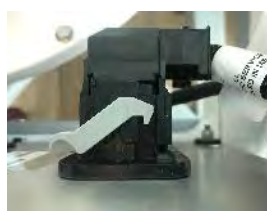
A properly connected GCM 70-pin connector
