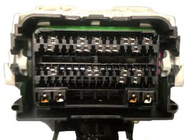
GCM 70-pin connector with face plate removed
