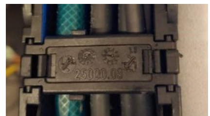
Figure 20: Properly secured chain link.
