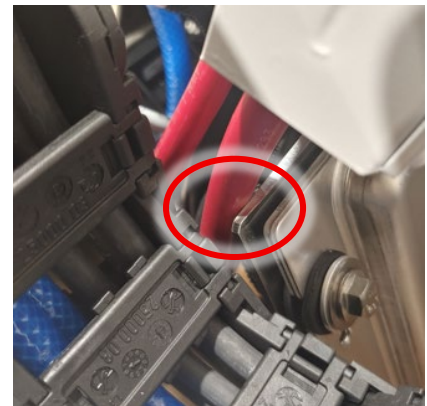
Figure 14: Seakeeper 1 area of cable chafing concern.
