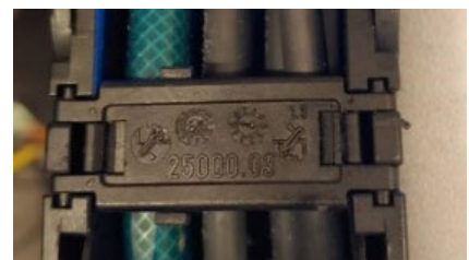
Figure 21: Properly secured chain link.
