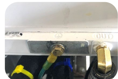
Figure 16: Motor drive ground connection
