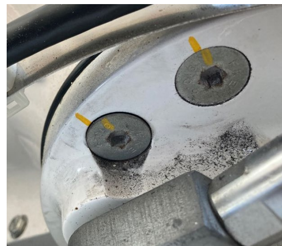
Figure 13: Yellow torque marks shown.
