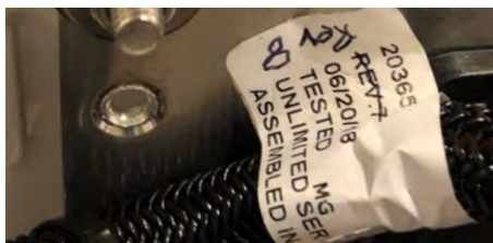
Seakeeper 2 harness should be Rev. 8 or later.
