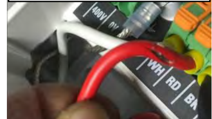
This damaged insulation caused DSPPF Fault in this Seakeeper.
