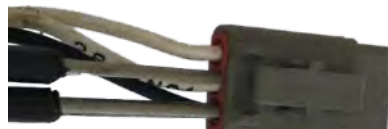
Deutsch plug with back probes inserted into pins 2 & 3.
