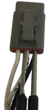
Angle sensor harness connector with back probes installed
