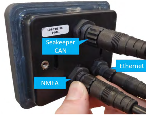
ConnectBox requires a SOG signal from NMEA network
