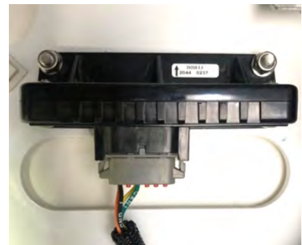
Seakeeper 18/16 IMU shown inside rear panel
