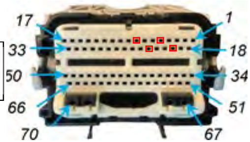
Testing continuity between pin 1 and GCM pin 5 (for Solenoid 1)
