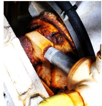
Seakeeper 3 with severe corrosion at rod end clevises, pins, and gimbal shafts
