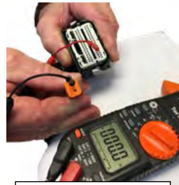
Testing continuity between pin 2 and GCM pin 4 (for Seakeeper 5, 6, or pump 2 on a Seakeeper 35/30HD/40)
