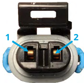
Figure 1: Seakeeper 9 bearing thermistor wire diagram (Other models similar)
