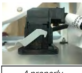
A properly connected GCM 70-pin connector
