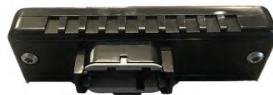
2 nd Generation IMU It will appear on info screen as "IMU: 2.X"
