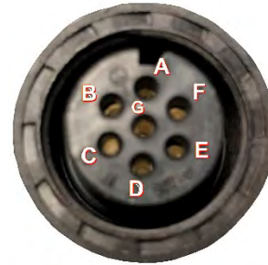
Proportional Brake valve connector for Seakeeper 26, 35, and 40.
