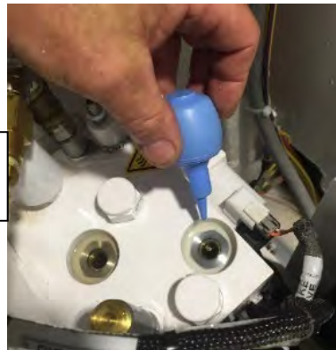
Bulb aspirator removing excess oil or debris in cavity.
