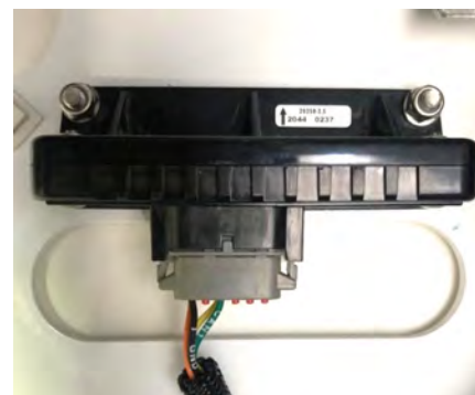
Seakeeper 18/16 IMU shown inside rear panel
