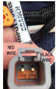
Low current DC input socket of harness
