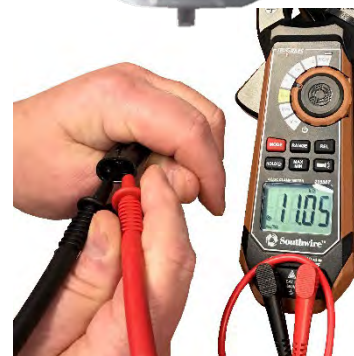
Meter in this photo is displaying 11.05 KΩ.
