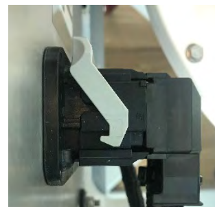
GCM connector fully inserted and locked
