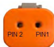
Deutsch connector to brake solenoid from wire harness
