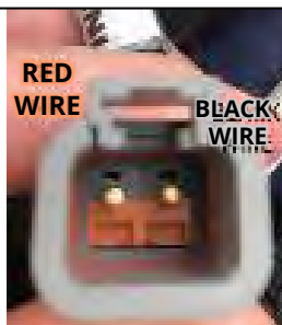
Close-up of the low DC input connector
