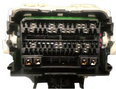
GCM 70-pin connector with face plate removed
