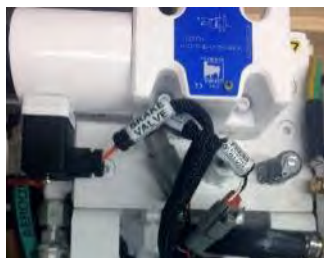
Seakeeper 16 Hirschmann plug shown on proportional valve
