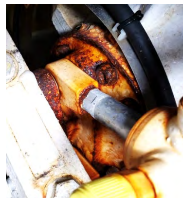
Seakeeper 3 with severe corrosion at rod end clevises, pins, and gimbal shafts
