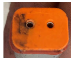
Evidence of moisture intrusion in a harness connector
